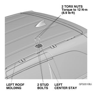
11. Place the left roof rail over the four remaining stud bolts.
