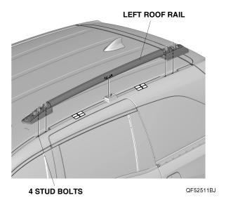
12. Install the four TORX nuts and two TORX bolts. Torque the TORX nuts to 12 N·m (8.9 lb·ft). Install the TORX bolts to 10 N·m (7.4 lb·ft).
