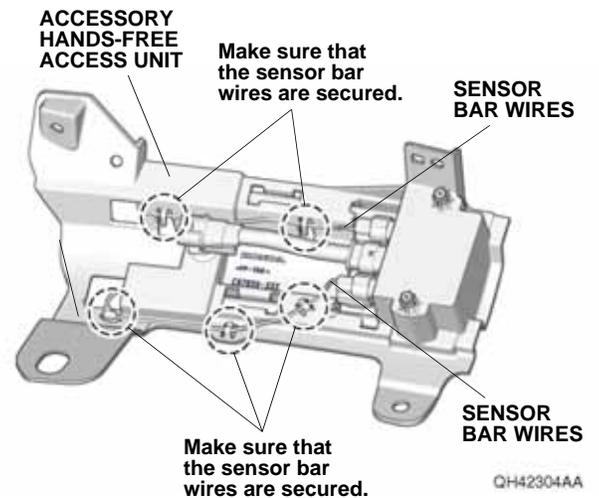
11. Install the accessory hands-free access unit to the trailer hitch cover. If the vehicle is equipped with the standard hands-free access power tailgate, use two self-tapping screws and one clip removed in step 6; if not, use new two self-tapping screws and one clip in the kit.
