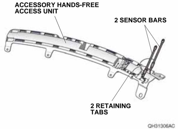
8. While wearing eye protection, use an air saw to cut the accessory hands-free access unit along the scribe line. Remove any burrs.
