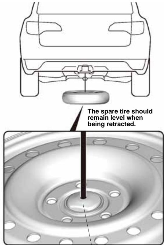
**The spare tire should remain level when being retracted.**
