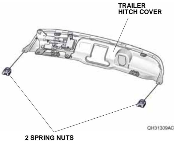
13. If equipped, plug the vehicle connector and secure the clip on the vehicle harness to the trailer hitch cover. Install the trailer hitch cover to the rear bumper with six retaining tabs, five clips, and the two bolts removed in step 5.
