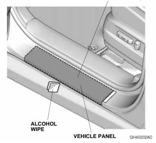
3. Using a spray bottle with the 3M protective tape application solution, spray the vehicle panel where the left front door sill protection film will attach. Then, spray some solution on your hands.
