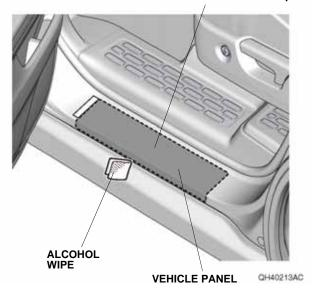
14. Using a spray bottle with the 3M protective tape application solution, spray the vehicle panel where the left rear door sill protection film will attach. Then, spray some solution on your hands.
