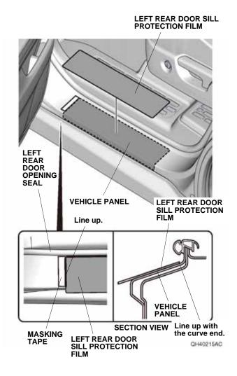
18. Starting from the inside and working outward, use the felt sleeve to smooth out the left and right sides of the upper section of the left rear door sill protection film. Move the felt sleeve in one direction only. If you see an air bubble, stop and gently peel up that section to work out the bubble. Work slowly, and keep pressure against the left rear door sill protection film.
