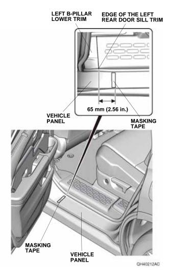
13. Using the alcohol wipe, thoroughly clean the vehicle panel where the left rear door sill protection film will attach.
