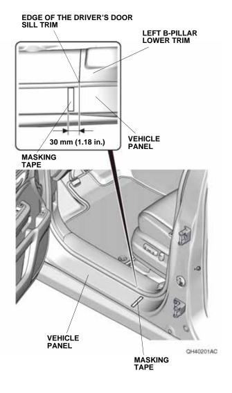
2. Using the alcohol wipe, thoroughly clean the vehicle panel where the left front door sill protection film will attach.
