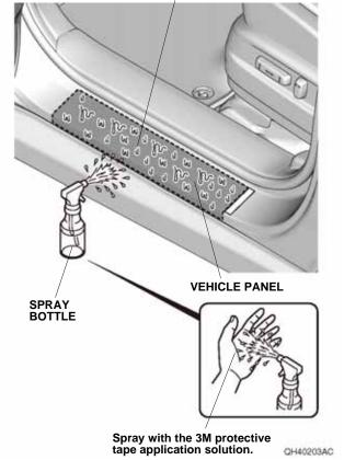
Remove the adhesive backings from the left front door sill protection film.
