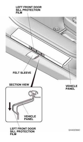
10. Starting from the center and working outward, use the felt sleeve to smooth out the left and right sides of the lower section on the left front door sill protection film. Move the felt sleeve in one direction only. If you see an air bubble, stop and gently peel up that section to work out the bubble. Work slowly, and keep pressure against the left front door sill protection film.
