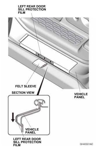
20. Repeat step 18 at the rear side of the lower section on the left rear door sill protection film.
