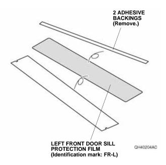
5. Spray the left front door sill protection film with the 3M protective tape application solution.
