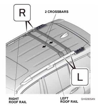
6. Line up the marks on the crossbars with the marks on the roof rails as shown. Tighten the eight thumbwheel screws to secure the crossbars to the roof rails.
