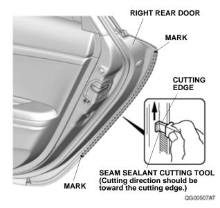
13. Apply touch-up paint to the cut seam sealant area, and let it dry.
