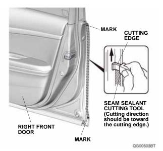
Apply touch-up paint to the cut seam sealant area, and let it dry.
