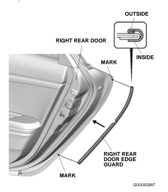
15. Starting at the character line, tap the right rear door edge guard into position with a series of light taps using a rubber mallet, then work up and down. Make sure the position of the right rear door edge guard is correct.
