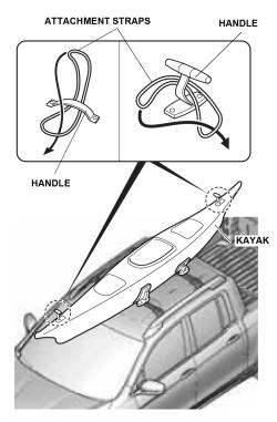
12. Attach one ratchet hook to the front attachment strap, and one ratchet hook to the rear attachment strap. Attach the front hook to the front bumper beam or tow hook. Attach the rear hook to the rear bumper beam or the trailer hitch. Secure the kayak to the vehicle by pulling the rope through the ratchet hooks.
