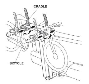
2. Install the two anti-sway cage assemblies to the bicycle arms as shown.
