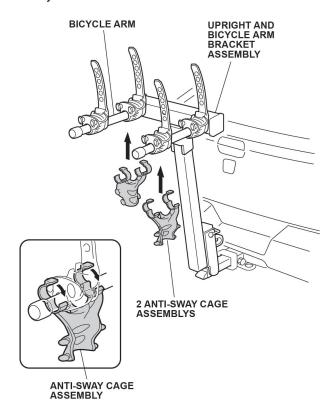
3. Tighten the bicycle arm straps securely around the bicycle frame.
