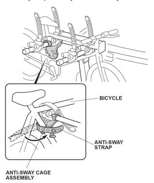
5. Using the strap provided, secure the bicycle wheels. Secure the strap buckle as shown.
