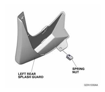
9. Install one spring nut on the left rear inner fender through the hole shown.
