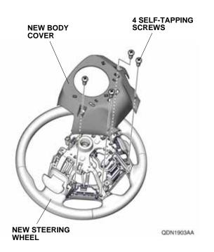
37. Secure the new cable reel cord and 4-pin connectors on the new body cover.
