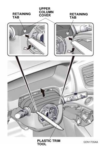
13. Release the upper column cover, and secure it to the dashboard with masking tape.
