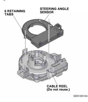
19. Install the steering angle sensor to the new cable reel with six retaining tabs.
