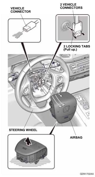
Remove the airbag. Do not drop the removed airbag or hit it on an object. Place the removed airbag in a safe place with the pad surface (top) facing upward.
