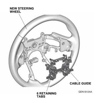
30. Install the new cable reel cord on the cable guide with one washer-screw. Plug the new cable reel cord 4-pin connector into the new steering wheel 4-pin connector, and secure the new cable reel cord to the cable guide.
