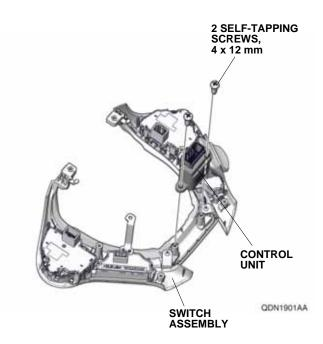
35. Plug the new cable reel cord connectors into the switch assembly, and install the switch assembly on the new steering wheel.
