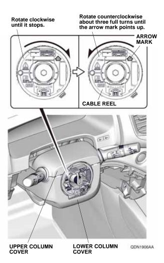
40. Before installing the steering wheel, make sure the front wheels are pointing straight ahead, then center the cable reel. Do this by first rotating the cable reel clockwise until it stops, then rotate it counterclockwise about three full turns. The arrow mark on the cable reel label should point straight up.
