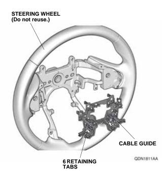
29. Install the cable guide on the new steering wheel with six retaining tabs.
