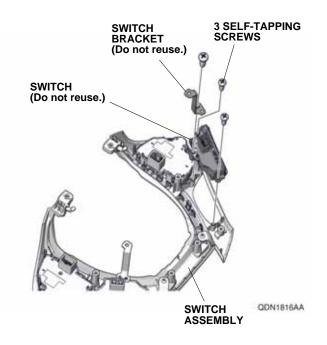
33. Install the new switch bracket and HSW switch on the switch assembly with three self-tapping screws.
