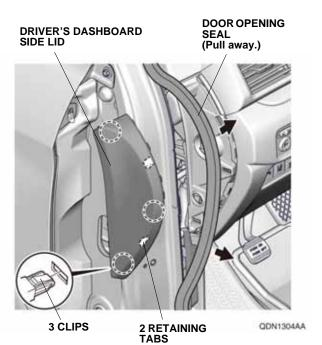
4. Remove the driver's dashboard under cover, unplug the vehicle connectors, and release the vehicle sensor.
