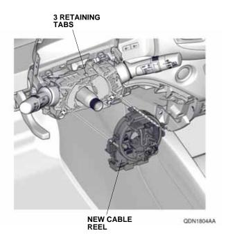
22. Plug the vehicle connectors into the new cable reel.
