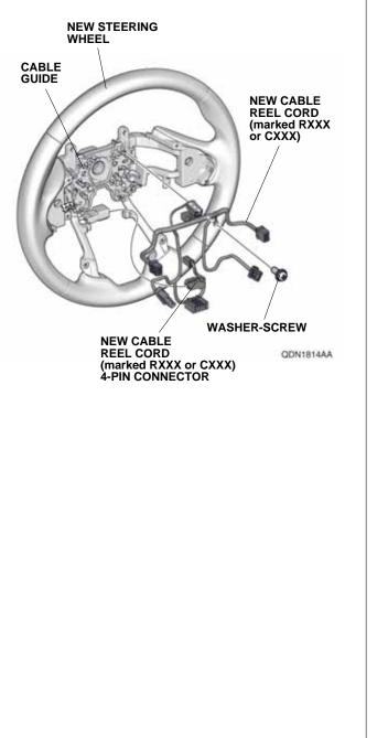
31. If equipped, install the left and right paddle shifters with two screws. Plug the new cable reel cord 4-pin connectors into the paddle shifter connectors, and secure the 4-pin connectors and paddle shifter cords on the cable guide.
