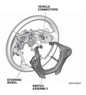
26. If equipped, remove the left and right paddle shifters and unplug the vehicle connectors.
