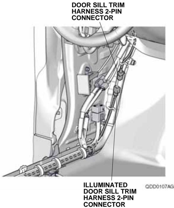
29. Bundle up the excess door sill trim harness and illuminated door sill trim harness, and secure them and 2-pin connectors to the vehicle harness with three wire ties.
