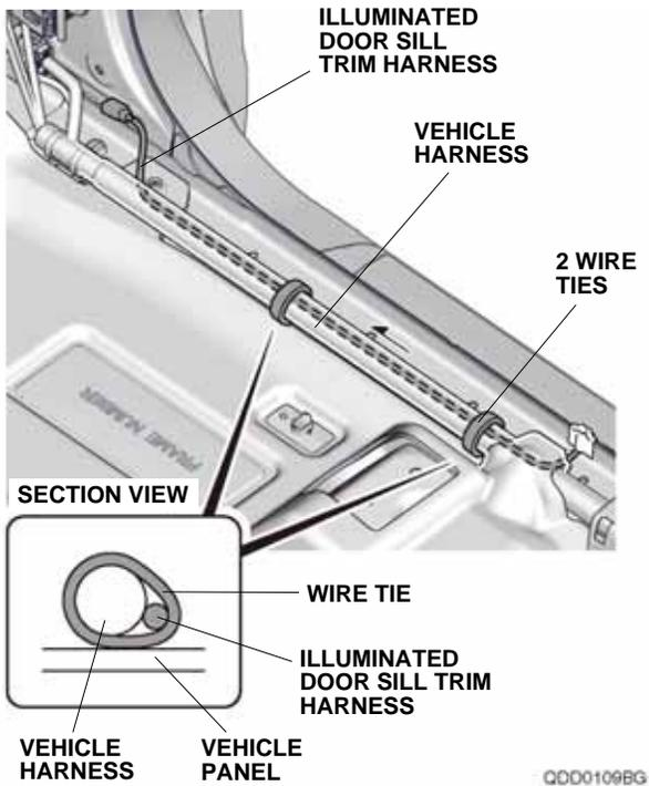
33. Secure the illuminated door sill trim harness to the vehicle harness with two wire ties.
