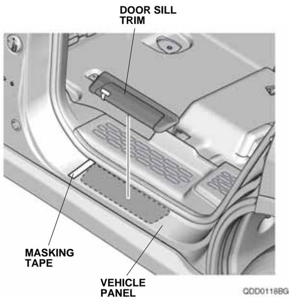
45. While applying light pressure against the door sill trim, carefully remove the adhesive backing.
