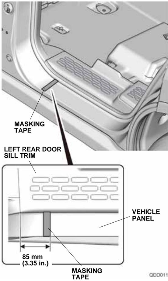
42. Using an alcohol swab, thoroughly clean the vehicle panel where the door sill trim will attach.
