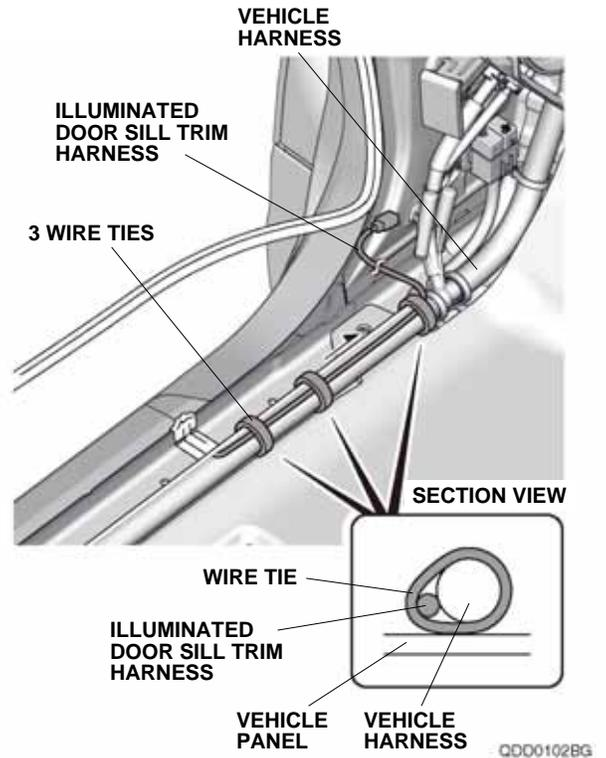
22. Secure the illuminated door sill trim harness to the vehicle harness with three wire ties.
