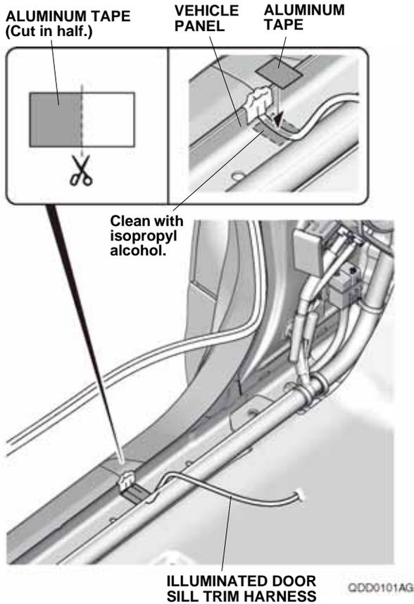
20. Using scissors, cut one aluminum tape in half. Secure the illuminated door sill trim harness to the vehicle panel with one half of aluminum tape.
