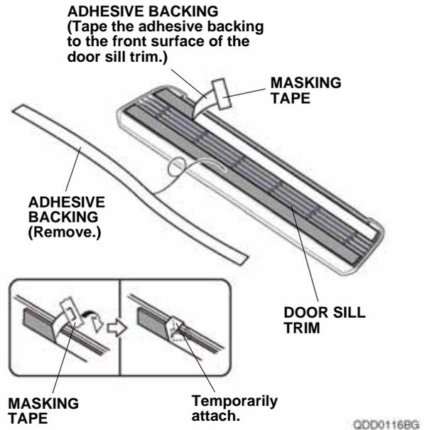
44. Line up the door sill trim with the masking tape and install the door sill trim to the vehicle panel.
