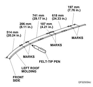
6. While wearing eye protection, use an air saw to cut the molding at the marks made in step 5. Remove any burrs.
