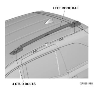
12. Install the four TORX nuts and two TORX bolts. Torque the TORX nuts to 12 N·m (8.9 lb·ft). Install the TORX bolts to 10 N·m (7.4 lb·ft).
