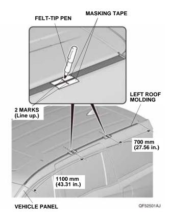
2. Using a plastic trim tool, carefully remove the left roof molding.
