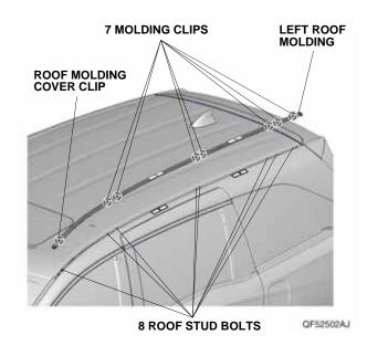
Using needle nose pliers, remove the seven molding clips and the roof molding cover clip from either the molding or the roof stud bolts.
