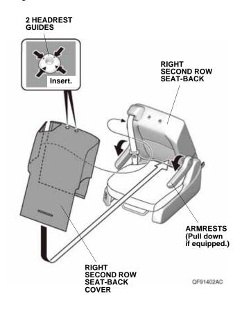
7. Secure the right second row seat-back cover with two fasteners.
