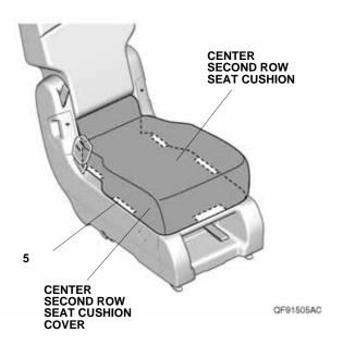
17. Secure the center second row seat cushion cover to the center second row seat cushion with one fastener. NOTE: Do not cover the anchor.
