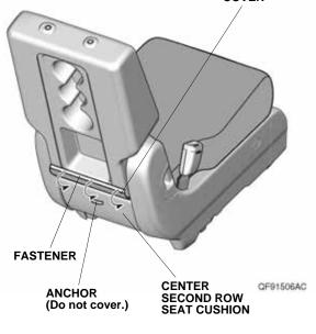
18. Fit the center second row seat-back cover to the center second row seat-back. Insert the center second row seat-back cover under each headrest guide.
