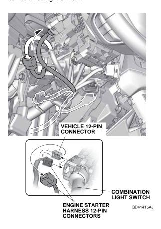
58. Align the white tape on the engine starter harness with the vehicle clip, and secure the engine starter harness and 12-pin connectors to the vehicle harness with one wire tie.
