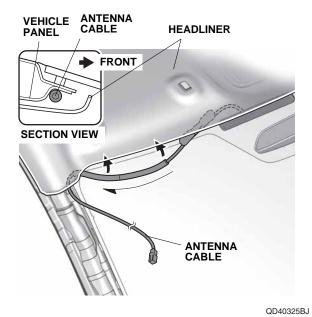
24. Route the antenna cable down the A-pillar as shown. Secure the antenna cable to the vehicle harness with four wire ties.
