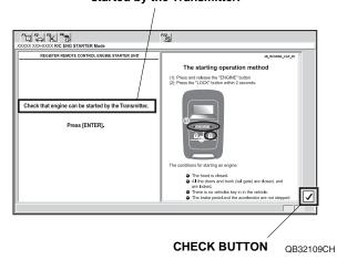
12. Perform the CHECK THE OPERATION OF THE REMOTE CONTROL ENGINE STARTER on page 26. Clear the DTCs, then disconnect the HDS/MVCI.
