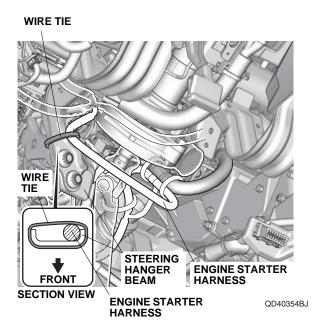
54. Route the engine starter harness along the vehicle harness. Align the white tape on the engine starter harness with end of the vehicle harness protector, and secure the engine starter harness to the vehicle harness with one wire tie.
