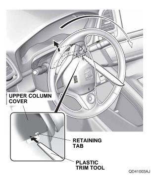
10. Turn the steering wheel 180° counterclockwise. Using a plastic trim tool, release the retaining tab.
