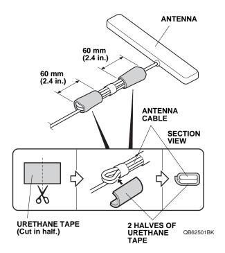
21. Using scissors, cut one urethane tape in half. Wrap two halves of urethane tape around the antenna cable at the measurement shown.
