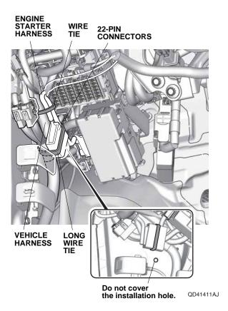
50. Route the engine starter harness as shown. Install the engine starter harness ground terminal with one ground bolt.
