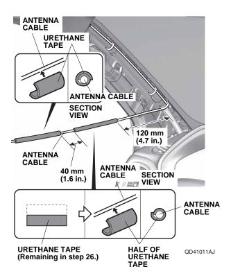
28. Pull away the door opening seal. Route the antenna cable down next to the dashboard, and tuck the antenna cable between the driver's A-pillar and the dashboard.
