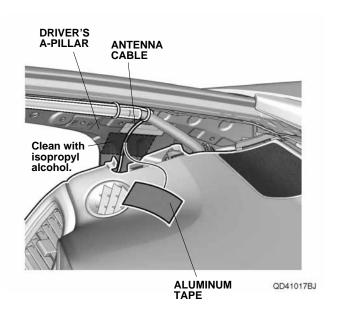
31. Attach the antenna cable to the driver's A-pillar with one aluminum tape.
