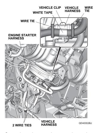
53. Secure the engine starter harness to the steering hanger beam with one wire tie.
