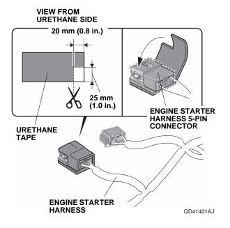
60. Unplug the vehicle 5-pin connector, and plug it into the engine starter harness 5-pin connector. Plug the remaining engine starter harness 5-pin connector into the vehicle 5-pin connector.
