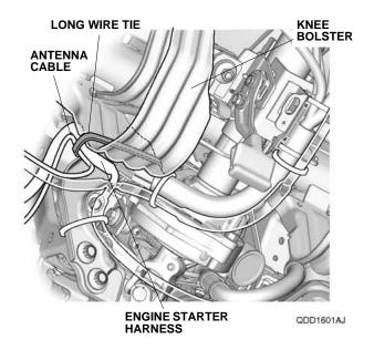
63. Align the white tape on the engine starter harness with the holes in the steering hanger beam, and secure the antenna cable and engine starter harness to the steering hanger beam with one wire tie.
