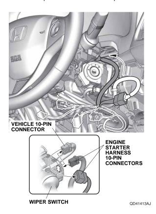
56. Align the white tape on the engine starter harness with the vehicle clip, and secure the engine starter harness and 10-pin connectors to the vehicle harness with one wire tie.
