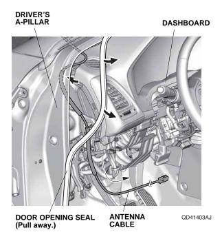
29. Secure the antenna cable to the steering hanger beam and vehicle harness with two wire ties.
