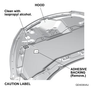
70. Remove the adhesive backing from the caution label, and attach the caution label to the hood as shown.
