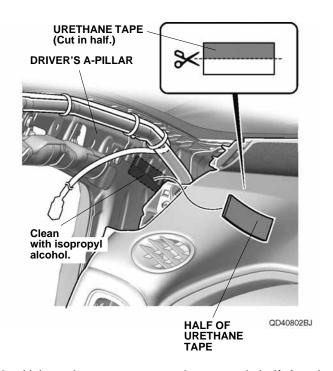
Using scissors, cut one urethane tape in half. Attach one half of urethane tape to the driver's A-pillar as shown. 27. Wrap the remaining urethane tape in step 26 and one urethane tape around the antenna cable of the measurements shown.
