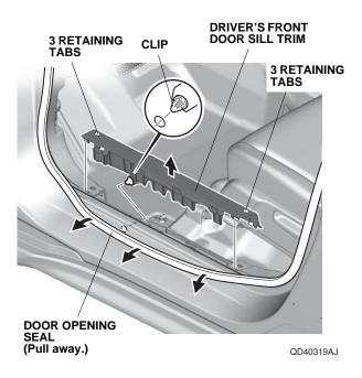
19. Pull away the door opening seal, and remove the driver's kick panel.
