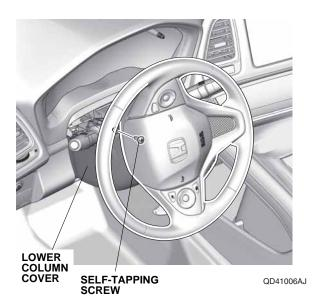
13. Turn the steering wheel 180° clockwise, and remove the self-tapping screw from the lower column cover.
