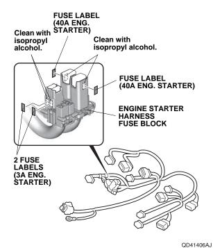
34. Attach four fuse labels to the engine starter harness fuse block.
