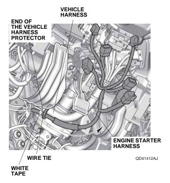
55. Unplug the vehicle 10-pin connector from the wiper switch, and plug it into the engine starter harness 10-pin connector. Plug the remaining engine starter harness 10-pin connector into the wiper switch.
