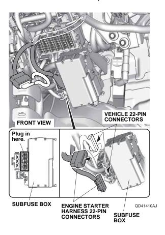
49. Secure the 22-pin connectors and engine starter harness to the vehicle harness with one wire tie and one long wire tie.
