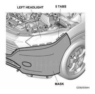
7. Attach nine hooks to the inside edge of the lower grille opening and front grille opening.
