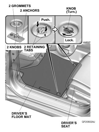
2. Place the grommets in the driver's floor mat over the anchors. Push the grommets into the anchors to secure the retaining tabs, then turn the knobs 90° to secure the floor mat.
