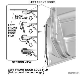
13. Using a shop towel, wipe the excess 3M protective tape application solution from the left front door edge film. Allow the left front door edge film to dry thoroughly.
