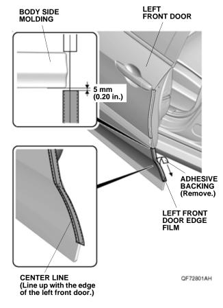
Line up the center line on the lower part of left front door edge film with the edge of the left front door. While applying light pressure, carefully remove the adhesive backing and attach the lower part of the left front door edge film to the left front door. 10. Insert the applicator into the soft sleeve. Starting from the top and working downward, use the soft sleeve to smooth the left front door edge film. Move the soft sleeve in one direction only.
