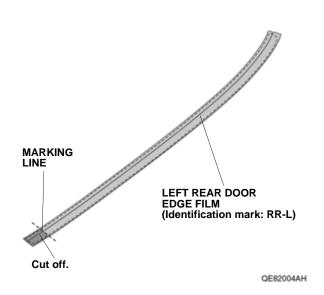
Open the left rear door. Peel back about 50 mm (1.97 in.) of adhesive backing from the left rear door edge film. Line up the V-notch with the bottom of the character line on the left rear door as shown.
