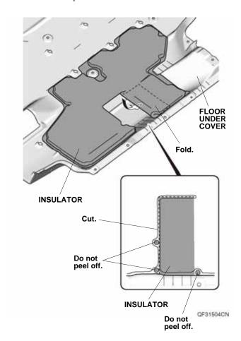
4. Using a utility knife, cut off the floor under cover as shown.
