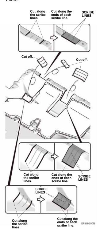
5. Using a utility knife, cut off the floor under cover as shown. Go to step 16.
