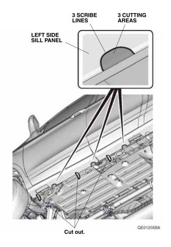
2. Remove the undercoating as shown. Apply touch-up paint where you removed the undercoating and allow it to dry thoroughly.
