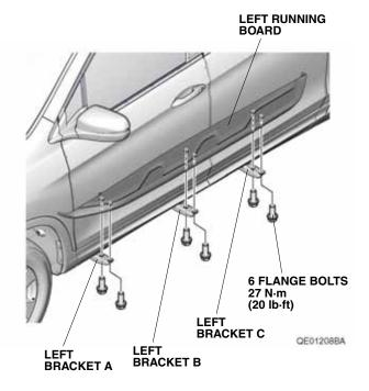
5. Tighten the six flange bolts loosely installed in step 3. Torque the flange bolts to 27 N·m (20 lb·ft).
