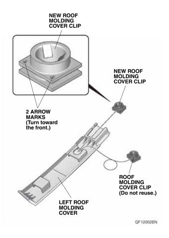
10. Install the left roof molding cover and left roof molding with the three molding clips and one roof molding cover clip. Align the marks made in step 1 on the vehicle panel and left roof molding.
