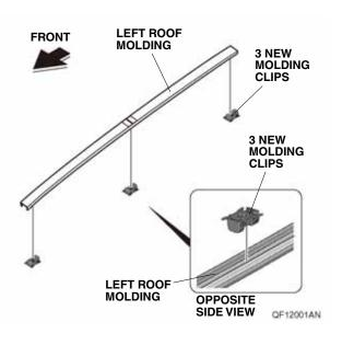
9. Remove the roof molding cover clip and install the new roof molding cover clip into the left roof molding cover as shown.
