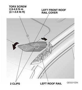
13. Install the left rear roof rail cover to the left roof rail with the two clips and one TORX screw. Torque the TORX screw to 2.9-4.9 N·m (2.1-3.6 lb·ft).
