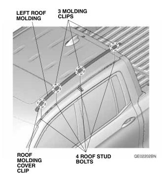
3. Remove the three molding clips from either the left roof molding or the roof stud bolts.
