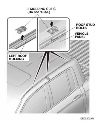
4. Remove any excess sealant from the four roof stud bolts.
