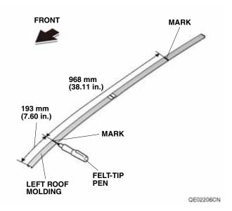
While wearing eye protection, use an air saw to cut the left roof molding at the two marks made in step 6. Remove any burrs.
