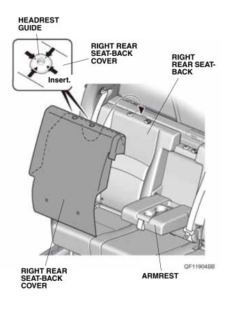
4. Insert the right rear seat-back cover and the three tabs into the right rear seat-back.
