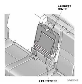
9. Pull down the armrest. Fit the left rear seat-back cover onto the left rear seat-back through the center seat belt. Insert the left seat-back cover under each headrest guide.
