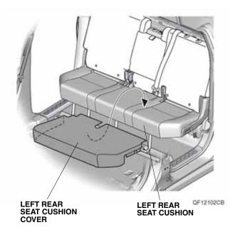
14. Raise the left rear seat cushion and secure the left rear seat cushion cover with the eight hooks and two tabs.
