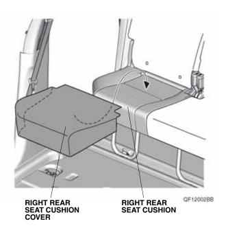
18. Raise the right rear seat cushion and secure the right rear seat cushion cover with the six hooks and two tabs.
