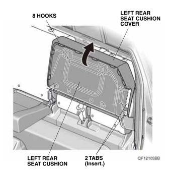
15. Secure the left rear seat cushion cover with the two fasteners.
