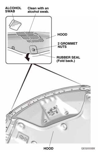
4. Using a felt-tip pen, make the two marks on the hood as shown.
