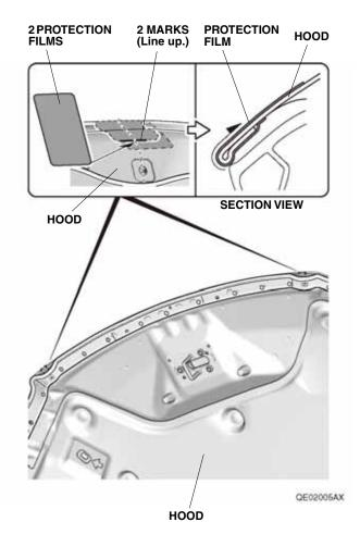
6. Close the hood. Using one alcohol swab, thoroughly clean the area where the hood protector will attach.
