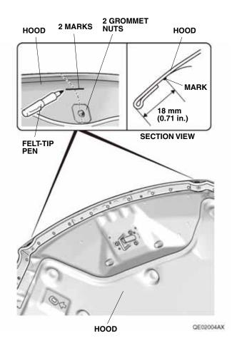
5. Remove the two adhesive backings from the two protection films and attach them as shown.
