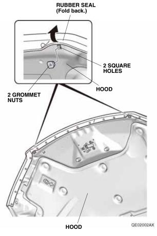
Open the hood. Fold back the rubber seal and locate the two square holes on the underside of the hood. Push one grommet nut into each square hole in the hood. 3. Fold back the rubber seal and using one alcohol swab, clean the areas of the hood where the two protection films will attach.
