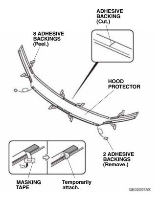
Attach a piece of masking tape to the end of the adhesive backings as shown. Peel back the adhesive backings partway and temporarily attach them to the front surface of the hood protector as shown. Remove the remaining adhesive backings. 10. Close the hood. Position the hood protector on the hood. Line up the holes in the hood protector with the holes in the two brackets and line up the hood protector with the hood edge.
