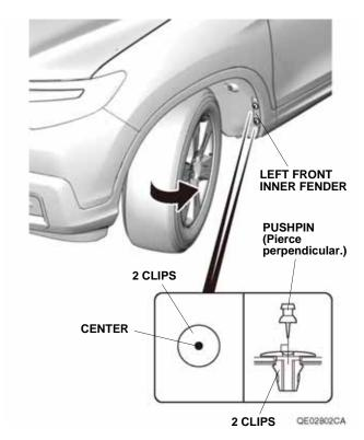
Using a pushpin, pierce the center of the top two clips on the left front inner fender.
