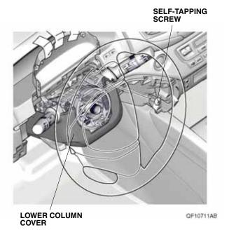
35. Turn the steering wheel 180° counterclockwise and remove the other self-tapping screw from the lower column cover.
