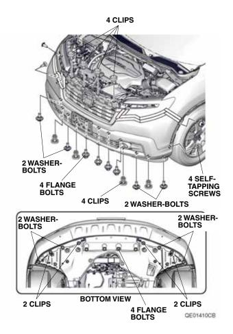
• With the help of an assistant, release the seven retaining tabs on each side.
