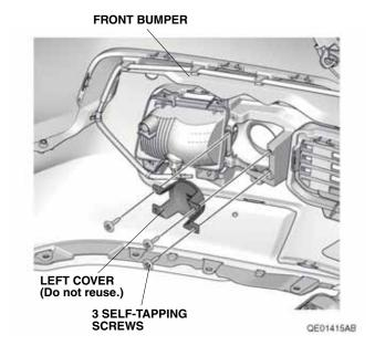
9. Install the left fog light on the front bumper with the three self-tapping screws removed in step 8.
