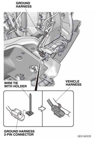
23. Secure the ground harness 2-pin connector to the vehicle harness with the wire tie installed in step 22. Reinstall the right front inner fender.
