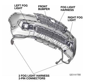
12. Secure the fog light harness to the two holes on the front bumper with two wire ties with clip on each side.
