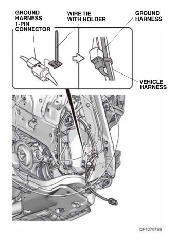
21. Secure the 1-pin connectors and ground harness to the vehicle harness with the wire tie installed in step 20.
