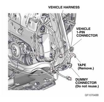
18. Plug the ground harness 1-pin connector into the vehicle 1-pin connector.
