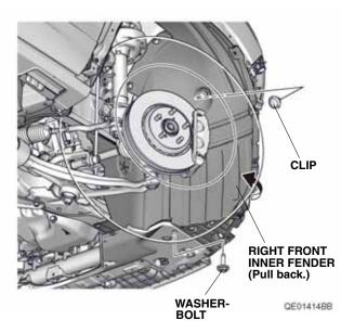
7. Remove one washer-bolt and one clip and pull back the right front inner fender as shown.
