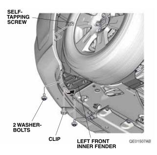
2. Insert your hand inside of the left front inner fender. Unplug the connector from the fog light.
