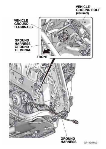
Route the ground harness along the vehicle harness and secure it to the vehicle harness with three wire ties.
