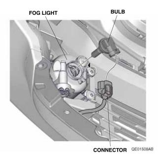
3. Remove the bulb from the fog light as shown. NOTE: Turn the fog light bulb counterclockwise.
