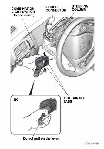
39. Push in on the two retaining tabs, slide the light switch out, and remove it from the steering column. Do not pull on the lever.
