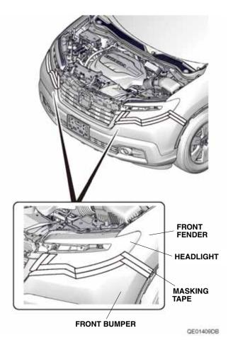
• Remove the four self-tapping screws, eight clips, four washer-bolts, and four flange bolts.
