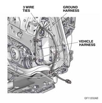
Locate the vehicle 1-pin connector taped to the vehicle harness. Remove the tape to free the vehicle 1-pin connector. Remove the dummy connector from the vehicle 1-pin connector.
