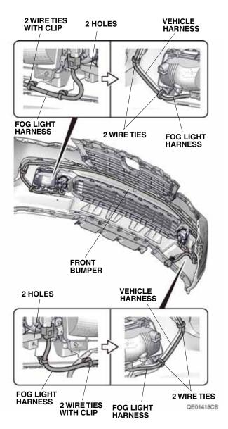
13. Secure the fog light harness to the vehicle harness with two wire ties on each side.
