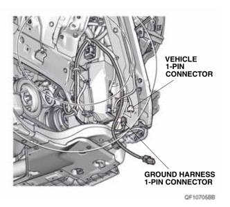
19. Secure the ground harness to the vehicle harness with three wire ties.
