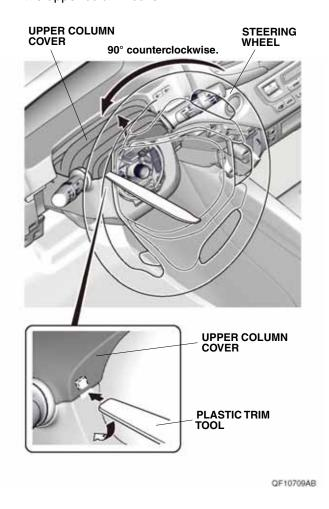
32. Turn the steering wheel 180° clockwise. Using a plastic trim tool, release the upper column cover.
