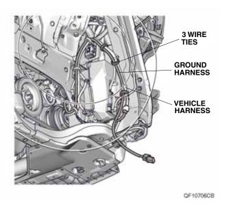
20. Install the wire tie with holder to the ground harness 1-pin connector.
