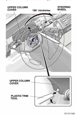
33. Release the upper column cover and secure it to the dashboard with masking tape.
