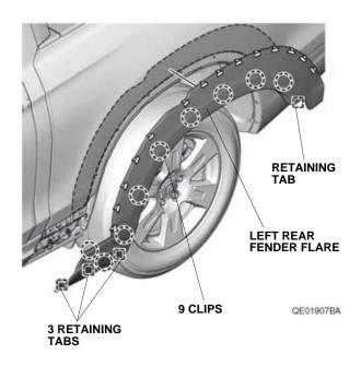
41. Secure the left rear fender flare to the left rear fender with the five self-tapping screws removed in step 34.
