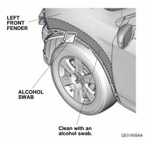
11. Install the left front fender flare to the left front fender.
