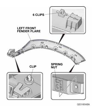
8. Install one spring nut to the left front fender flare as shown.
