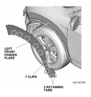
12. Secure the left front fender flare to the left front fender with the two self-tapping screws removed in step 2.
