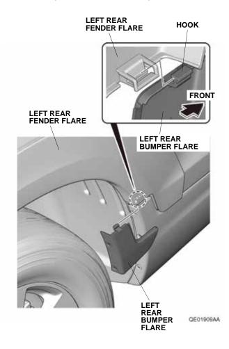
45. Secure the left rear bumper flare to the rear bumper with the two remaining self-tapping screws removed in step 34.
