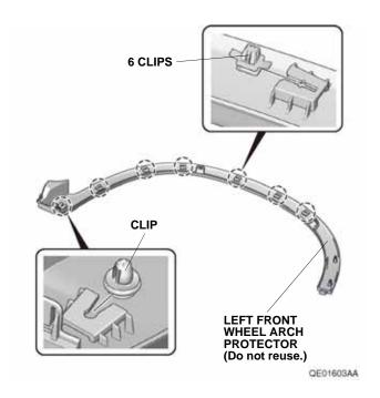
7. Install the seven clips removed in step 6 to the left front fender flare.
