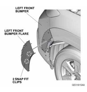
28. Pull back the left front inner fender. Secure the left front bumper flare to the front bumper with the four clips.
