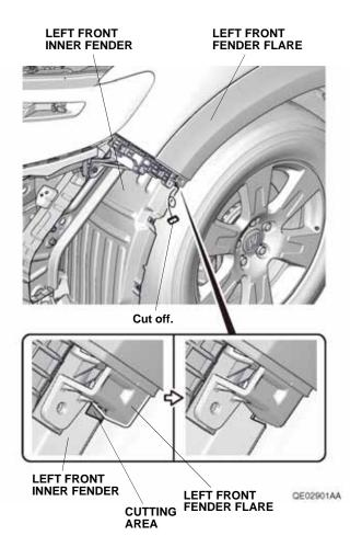
16. Secure the left front fender flare to the vehicle bracket with the self-tapping screw removed from the front bumper.
