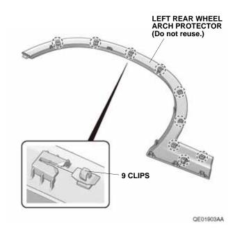
37. Install the nine clips removed in step 36 to the left rear fender flare.
