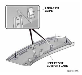
25. Attach a piece of masking tape to the end of the adhesive backings as shown. Peel back the adhesive backings partway and temporarily attach them to the front surface of the left front bumper flare.
