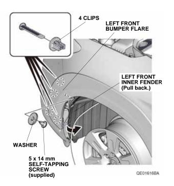
29. Secure the left front bumper flare to the front bumper with one washer and one 5 x 14 mm self-tapping screw.
