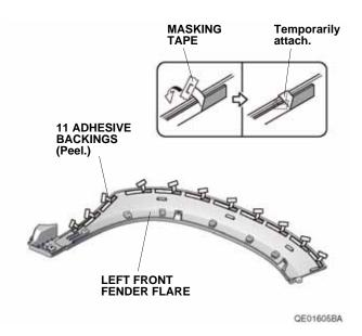
10. Using one alcohol swab, thoroughly clean the area where the left front fender flare will attach.
