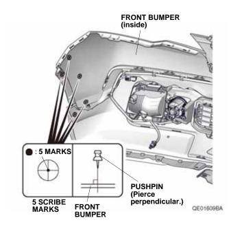
19. While wearing eye protection, drill the four pierced marks on the front bumper to 10 mm. Drill first with a 3 mm drill bit. Next, drill with a 6 mm drill bit and an 8 mm drill bit. Then, finish with a 10 mm drill bit. Remove any burrs.
