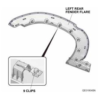
38. Attach a piece of masking tape to the end of the adhesive backings as shown. Peel back the adhesive backings partway and temporarily attach them to the front surface of the left rear fender flare. Remove the remaining adhesive backings.
