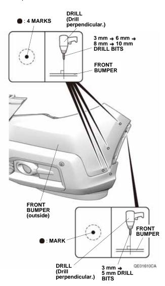
While wearing eye protection, drill one pierced mark to 5 mm. Drill first with a 3 mm drill bit, then finish with a 5 mm drill bit. Remove any burrs. NOTE: Make sure to drill perpendicular to the front bumper. 21. While wearing eye protection, cut off the front bumper along the scribe line with an air saw. Remove any burrs.
