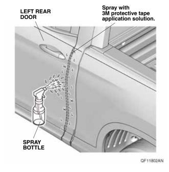
15. Open the left rear door again. Peel back about 50 mm (1.97 in.) of adhesive backing from the left rear door edge film. Align the V-notch in the left rear door edge film with the character line of the left rear door.
