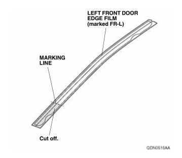
Open the left front door again. Peel back about 50 mm (1.97 in.) of adhesive backing from the left front door edge film. Align the V-notch in the left front door edge film with the character line of the left front door.
