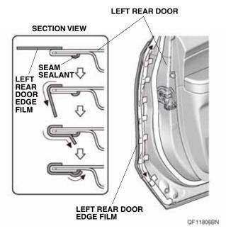
Using a shop towel, wipe the 3M protective tape application solution from the left rear door edge film.
