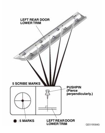
19. While wearing eye protection, drill the five pierced marks to 7 mm. Drill first with a 3 mm drill bit, then finish with a 7 mm drill bit. Remove any burrs. NOTE: Make sure to drill perpendicularly to the left rear door lower trim.
