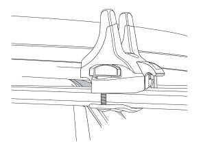
6. Slide the buckle on an attachment strap into the clip on the base.
