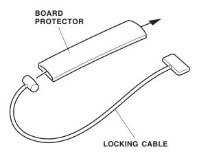
14. Insert the locking cable plate into the slit in each snowboard carrier. To carry one snowboard, insert the plate into the lowest slit. To carry two snowboards, use one of the upper three slits in the carrier.
