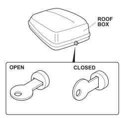
**Locking:** Press down on the lid. You should hear a click. Be sure the lid is latched by attempting to lift the lid. Turn the key clockwise to lock the roof box. Remove the key while not in use. Be sure the straps are not outside the roof box.
