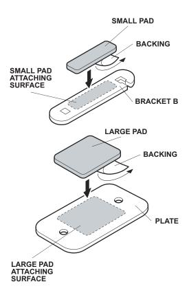
Using isopropyl alcohol on a shop towel, clean four plates where the large pads will attach. Remove the backing from the large pads and attach them to the plates. 4. Under the roof box, insert a bolt through bracket B, through the plate, and into the predrilled hole in the bottom of the roof box.
