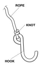
10. Route the other end of the rope through the bottom of the ratchet hook in the direction shown, and turn the spool until the rope end comes out of the ratchet.
