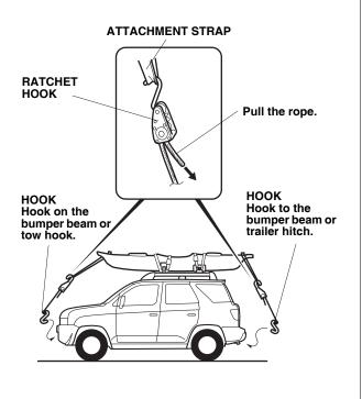
13. To loosen the rope, push up on the ratchet strap lever, then pull the rope.
