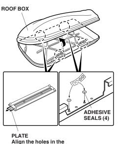
Align the holes in the plate with the front crossbar.
