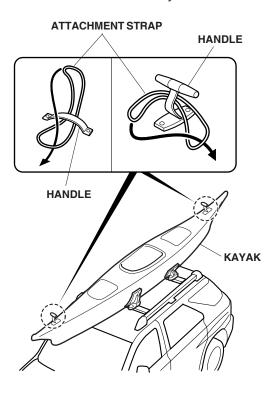
12. Attach one ratchet hook to the front attachment strap, and one ratchet hook to the rear attachment strap. Attach the front hook to the front bumper beam or tow hook. Attach the rear hook to the rear bumper beam or the trailer hitch. Secure the kayak to the vehicle by pulling the ropes through the ratchet hooks.
