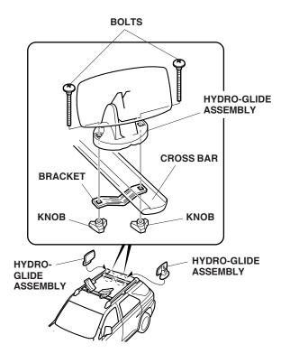
3. Rest the front of the kayak on the hydro-glide assemblies. Standing behind or alongside the kayak, lift up the rear of the kayak and push it forward, sliding it on the hydro-glide assemblies and saddles. Make sure the kayak reaches the front saddles before you lower it.
