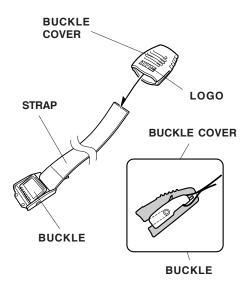
7. Route the strap under the front crossbar, and around the kayak as shown. Slide the buckle cover away from the buckle, route the strap through the buckle, and tighten the strap. Slide the buckle cover back over the buckle.
