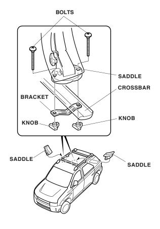
Position the two hydro-glide assemblies on the rear crossbar. Loosely install the hydro-glide assemblies with one bracket, two bolts, and two knobs for each assembly. The distance between the two assemblies should be the same as the width of the kayak.
