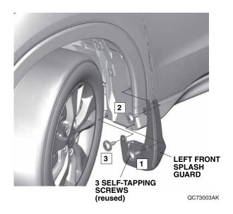
4. Remove the two self-tapping screws.
