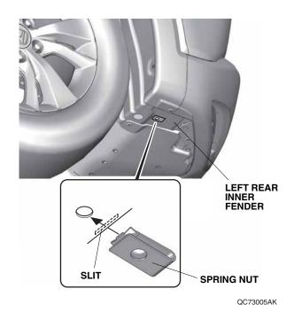
Secure the left rear splash guard with two 5 x 25 mm self-tapping screws and one 5 x 18 mm self-tapping screw in the order shown below.
