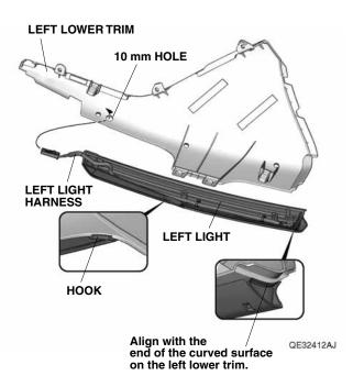
33. Secure the left light to the left lower trim with three self-tapping screws.
