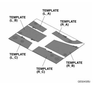
15. Attach the templates to the left lower trim with masking tape.
