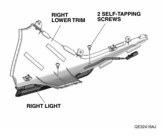
38. Using isopropyl alcohol on a shop towel, thoroughly clean the right lower trim where the aluminum tape will attach.
