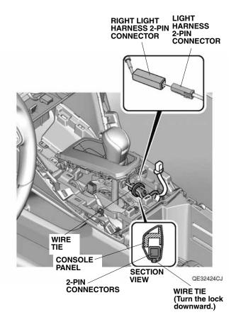
50. Plug the left light harness 2-pin connector into the light harness 2-pin connector.
