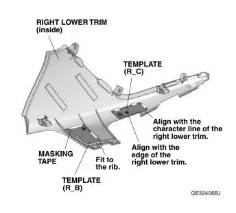
22. Using a pushpin, pierce the center of three marks on the templates.
