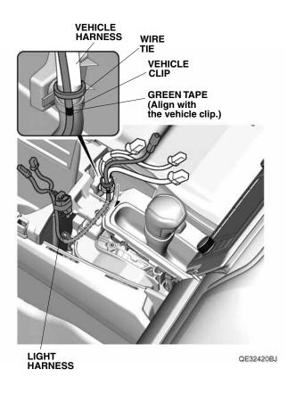
45. Secure the light harness 2-pin connector to the vehicle harness with one wire tie.
