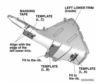
16. Using a pushpin, pierce the center of four marks on the templates.
