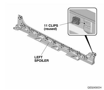
13. Install the left spoiler on the vehicle panel.
