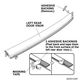
16. Remove the adhesive backing.
