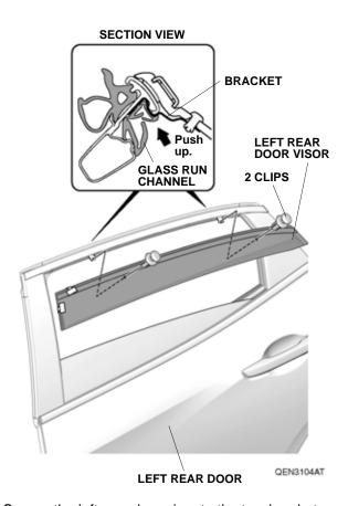
18. Secure the left rear door visor to the two brackets with the two clips. Make sure to push up on the brackets while installing the two clips. NOTE: Be extremely careful when installing the clips; they cannot be reinstalled after installation.
