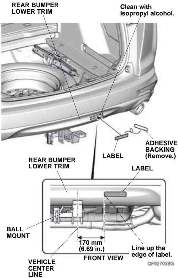
88. Remove the adhesive backing from the label, and attach the label to the rear bumper lower trim as shown.
