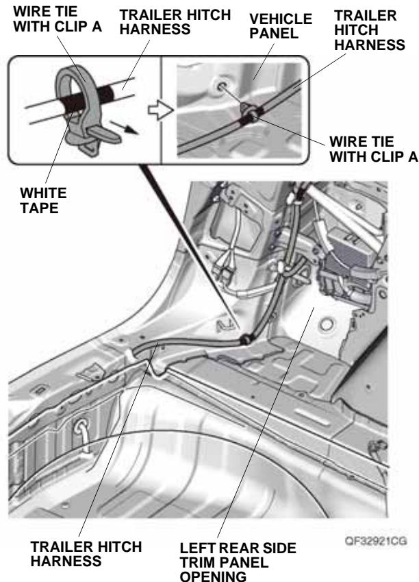
78. Peel back the floor carpet, then route the trailer hitch harness as shown.
