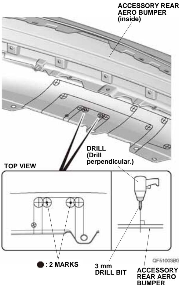
42. While wearing eye protection, enlarge the 3 mm holes to 20 mm using a 20 mm hole saw. Remove any burrs.
