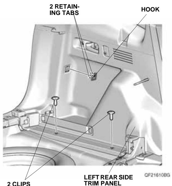
13. Pull away the door opening seal and weatherstrip from around the left rear side trim panel. Remove the left rear side trim panel, and unplug the vehicle connector.
