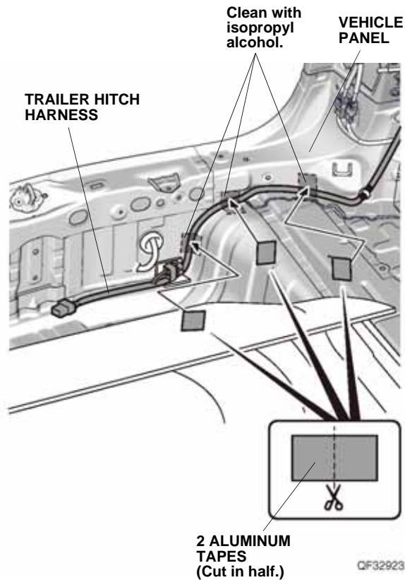
81. Using scissors, cut two aluminum tapes in half, and secure the trailer hitch harness to the vehicle panel with three halves of aluminum tape as shown.
