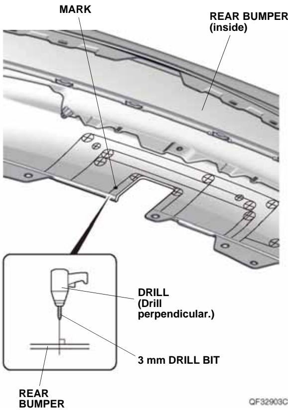
38. While wearing eye protection, enlarge the 3 mm hole to 14 mm using a 14 mm hole saw. Remove any burrs.
