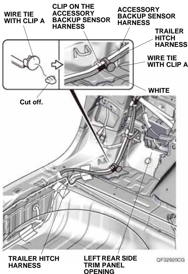
76. Line up the white tape on the trailer hitch harness to the clip on the accessory backup sensor harness, and secure the trailer hitch harness to the accessory backup sensor harness with one wire tie with clip A. Go to step 78.
