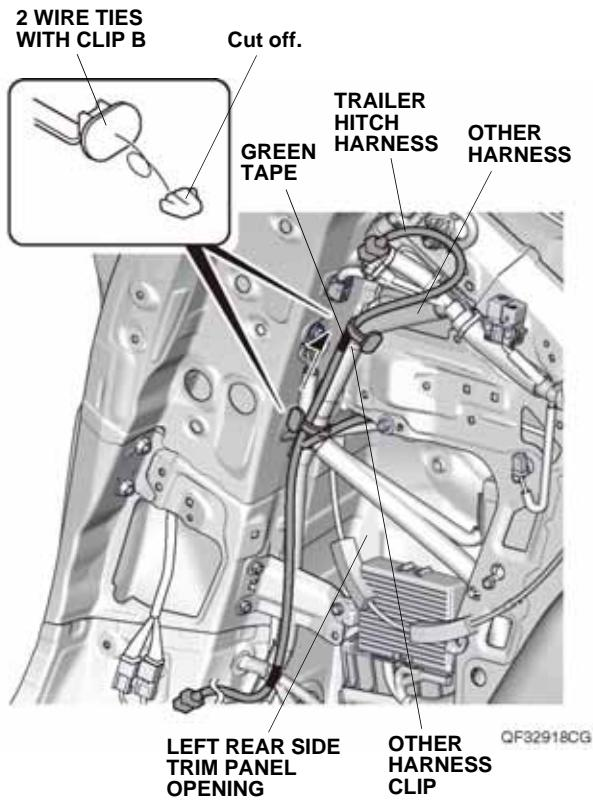
68. Using diagonal cutters, cut off the clip portion off of two wire ties with clip B.
