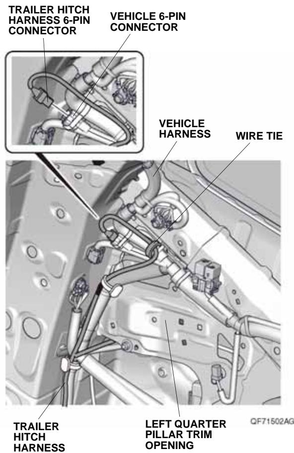
74. Secure the trailer hitch harness to the vehicle harness with one wire tie.
