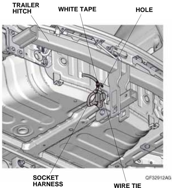
61. Remove the vehicle grommet. Route the socket harness through the vehicle panel hole.
