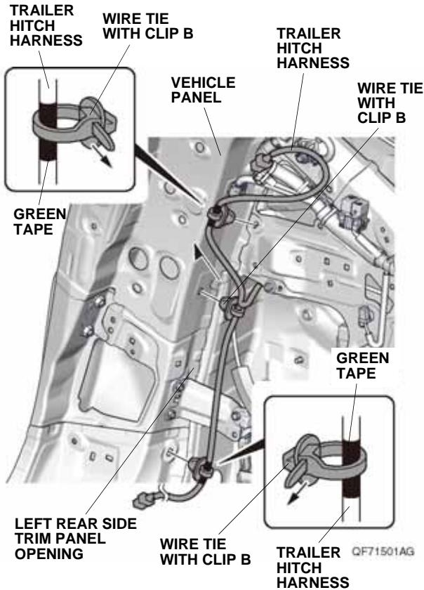
72. Secure the trailer hitch harness to the vehicle panel with one wire tie with clip B.
