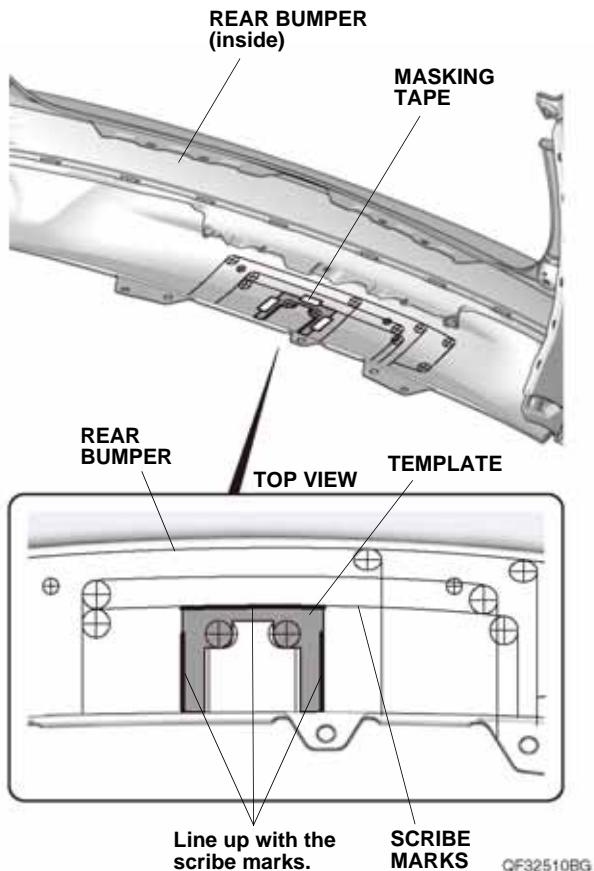
30. Using a felt-tip pen, mark the rear bumper along the template.
