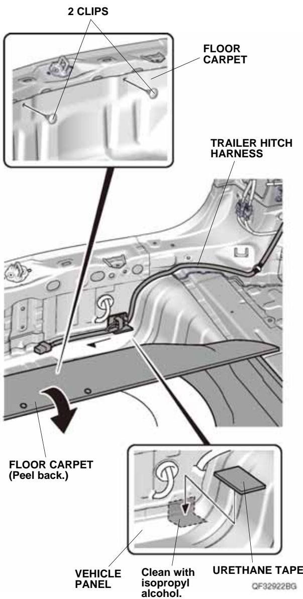
79. Using isopropyl alcohol on a shop towel, thoroughly clean the vehicle panel where the urethane tape will attach. Attach the urethane tape to the vehicle panel as shown.
