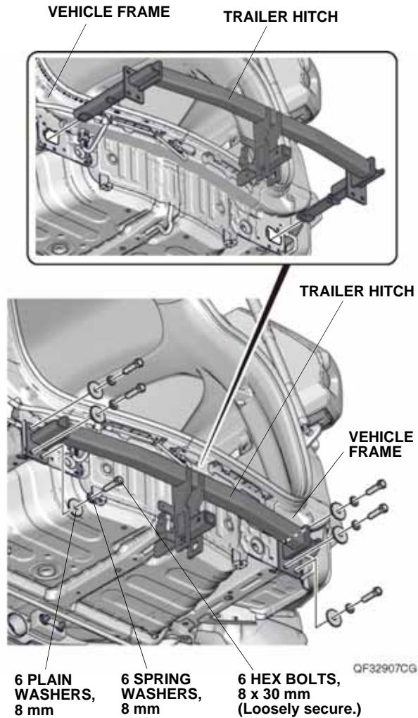
53. Loosely secure the trailer hitch to the vehicle frame with six 8 mm plain washers, six 8 mm spring washers, and six 8 x 30 mm hex bolts.
