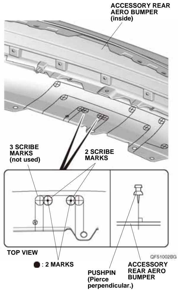
41. While wearing eye protection, drill the two pierced marks on the accessory rear aero bumper with a 3 mm drill bit.
