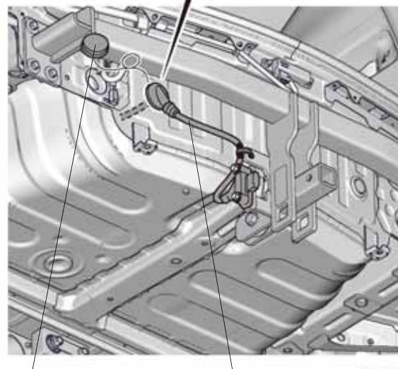
62. Install the grommet on the socket harness into the vehicle panel hole.
