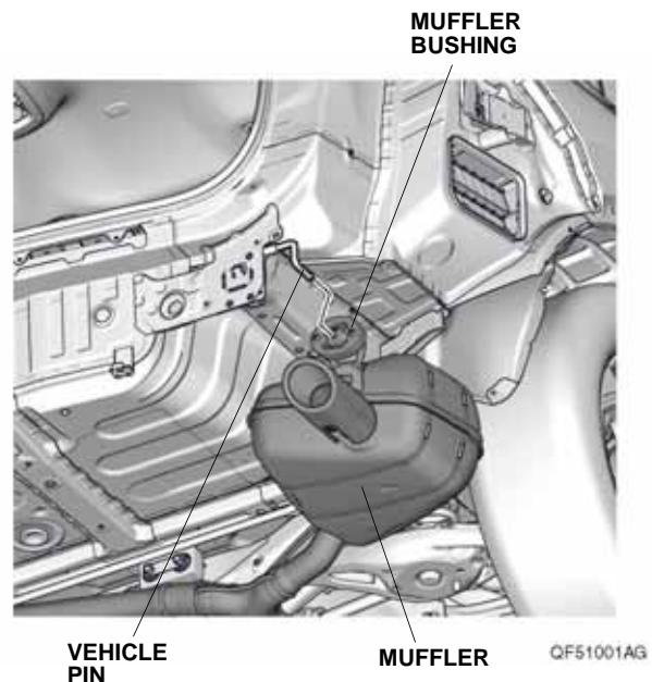
26. Remove the muffler bushing from the left side of the vehicle the same way, if equipped.
