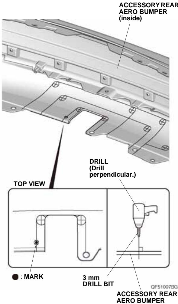
46. While wearing eye protection, enlarge the 3 mm hole to 14 mm using a 14 mm hole saw. Remove any burrs.
