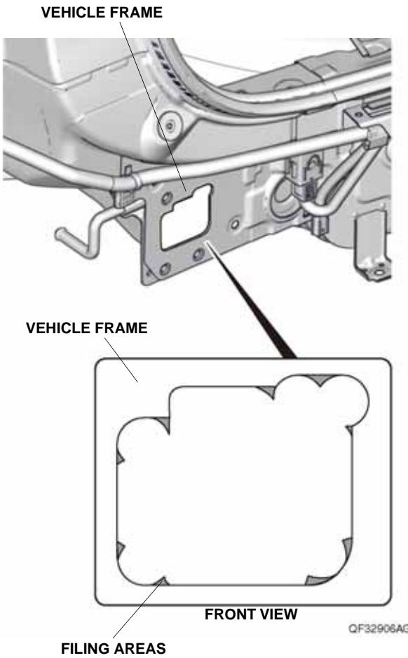
50. Apply touch-up paint to the edges of the holes. Allow the touch-up paint to dry before proceeding to the next step.
