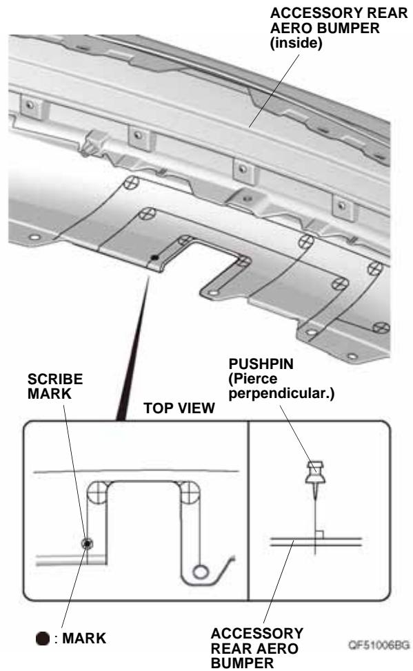
45. While wearing eye protection, drill the pierced mark on the accessory rear aero bumper with a 3 mm drill bit.
