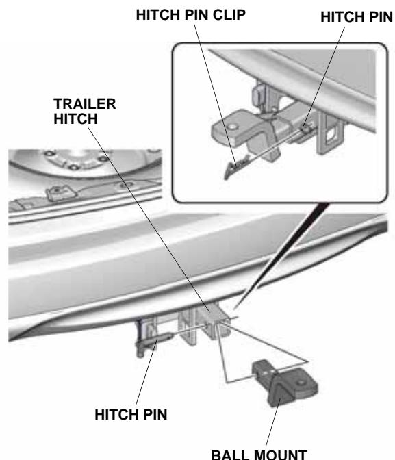
86. Secure the ball mount to the trailer hitch with the hitch pin and hitch pin clip.
