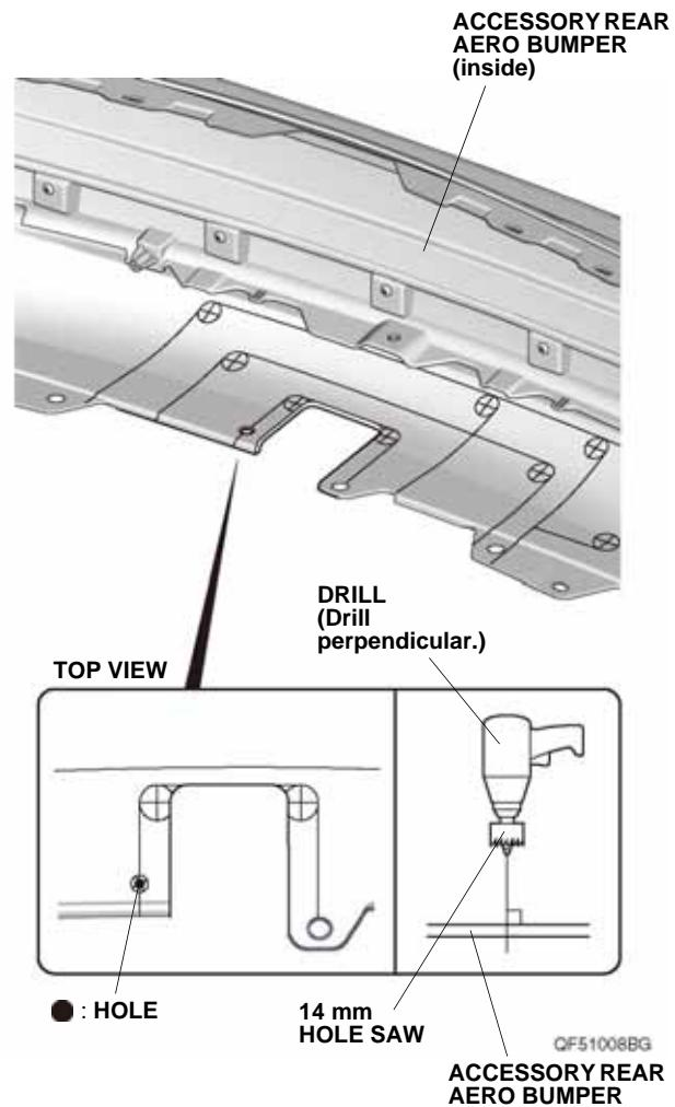
47. Install the hands free access unit to the accessory rear aero bumper with two self-tapping screws, four clips, and one bumper clip.
