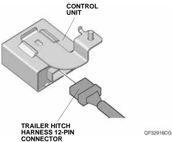
66. Install the control unit bracket to the vehicle panel with one 6 mm flange nut and one 6 mm plain washer.
