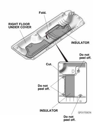
10. Using a utility knife, cut off the right floor under cover as shown.
