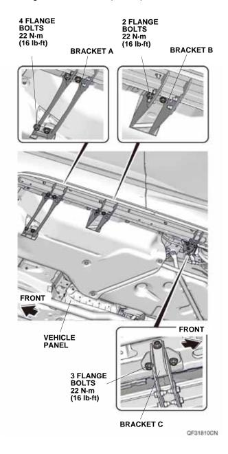
28. Secure the left running board to bracket A, bracket B, bracket C, and left bracket D with 13 flange bolts. Torque the flange bolts to 22 N·m (16 lb·ft).
