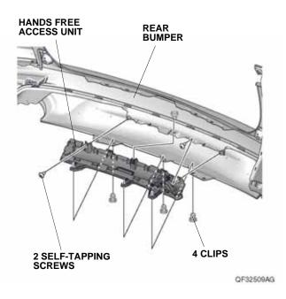
10. Remove the left rear upper bumper from the rear lower bumper. Repeat for the right rear upper bumper.
