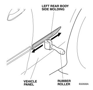
18. Turn the front and rear templates over, and repeat steps 1 through 17 to install the body side moldings on the right side of the vehicle.
