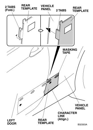
Insert the folded tabs of the rear template into the opening between the left door and the vehicle panel. Align the template with the character line, and tape the template to the vehicle panel with strips of masking tape. 5. Check that the edges of the front and rear templates are aligned. Readjust the templates if necessary.
