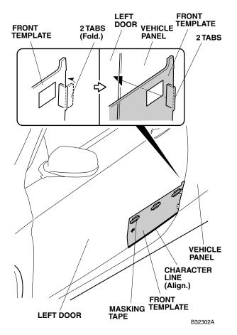
Insert the folded tabs of the front template into the opening between the left door and the vehicle panel. Align the template with the character line, and tape the template to the door with strips of masking tape. 3. Get the rear template. Fold the two tabs on the template in the direction shown.
