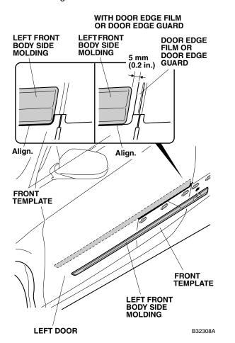
9. While applying light pressure against the left front body side molding, carefully remove the taped adhesive backings. Remove about 50 to 100 mm (2.0 to 4.0 in.) at a time.
