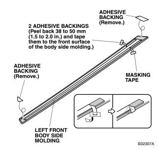
8. Align the left front body side molding with the front template, and attach it to the left door as shown. NOTE: If the vehicle is equipped with a door edge film or a door edge guard, attach the left front body side molding at the measurement shown.
