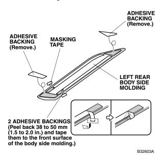
13. Align the left rear body side molding with the rear template, and attach it to the vehicle panel as shown.
