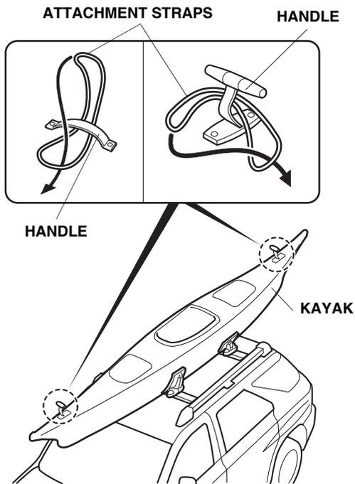
12. Attach one ratchet hook to the front attachment strap, and one ratchet hook to the rear attachment strap. Attach the front hook to the front bumper beam or tow hook. Attach the rear hook to the rear bumper beam or the trailer hitch. Secure the kayak to the vehicle by pulling the rope through the ratchet hooks.
