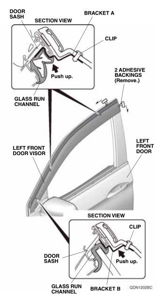
12. Using the palm of your hand, firmly press the left front door visor against the door sash.
