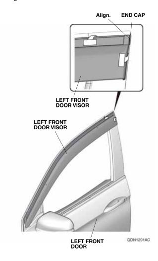
11. While applying light pressure against the left front door visor, carefully remove the taped adhesive backings. Make sure to push up on the brackets A and bracket B while removing the adhesive backings.
