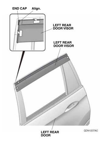
22. While applying light pressure against the left rear door visor, carefully remove the taped adhesive backings. Make sure to push up on the two brackets A while removing the adhesive backings. NOTE: While removing long top piece of adhesive backing, make sure that left rear door visor is positioned so that top edge of vehicle chrome is hidden by left rear door visor.
