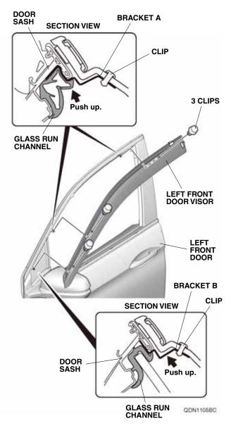
9. Secure the left front door visor to two brackets A and one bracket B with three clips. Make sure to push up on the two brackets A and one bracket B while installing the clips.
