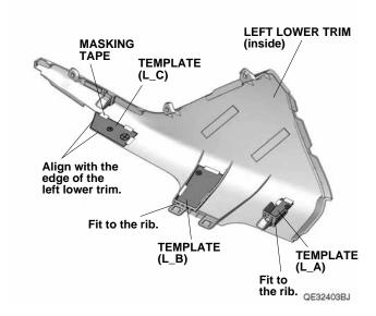
16. Using a pushpin, pierce the center of four marks on the templates.
