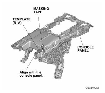
28. Using a pushpin, pierce the center of the mark on the template.
