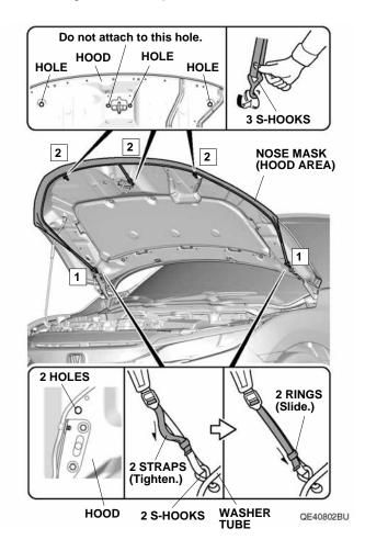
2. Attach three S-hooks to the underside of the hood by inserting your finger into the belt of each hook.
