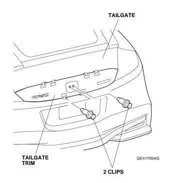
12. While applying light pressure to the tailgate trim, carefully remove the taped adhesive backings in the order shown.
