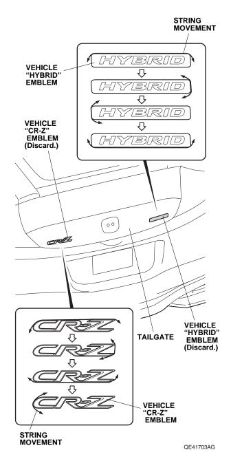
5. If the clips on the vehicle "H" emblem remained on the vehicle, use a needle nose pliers to remove the clips.
