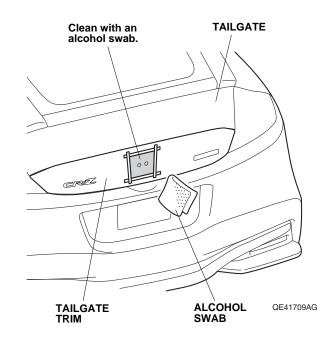
18. Remove the adhesive backing from the "H" emblem. Align the "H" emblem with the masking tape attached in step 15 and attach it to the tailgate trim.
