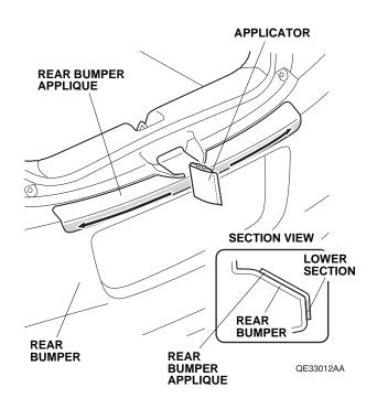
11. Using a shop towel, wipe the excess 3M protective tape application solution from the rear bumper applique.
