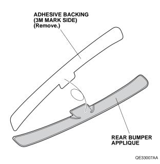
4. Using a spray bottle with 3M protective tape application solution, spray the rear bumper applique as shown.
