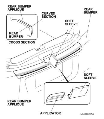
7. Starting from the center and working outward, use the applicator and soft sleeve to smooth out the curve end section of the rear bumper applique against the rear bumper.
