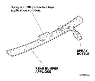
5. Align the end of the rear bumper applique with the character line, and attach it to the rear bumper.
