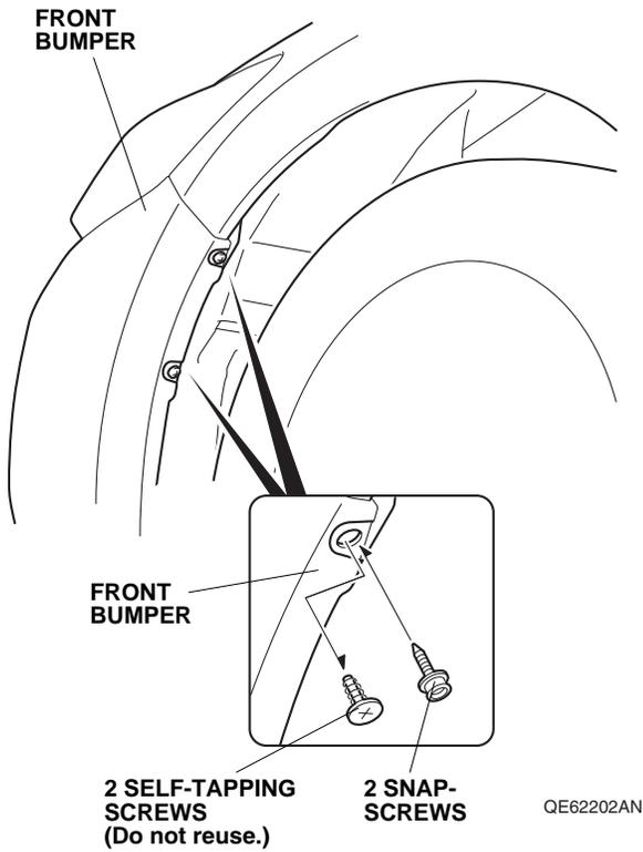
2. Remove and discard the two self-tapping screws from the front bumper.
