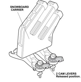
5. Attach the two bottom clamps to the top clamps.
