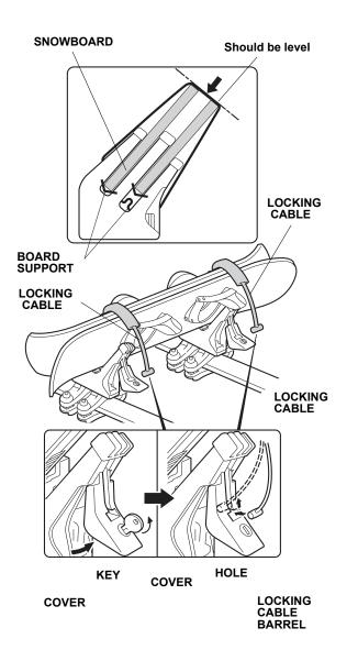
15. Check that the locking cables are installed securely, then close the covers.
