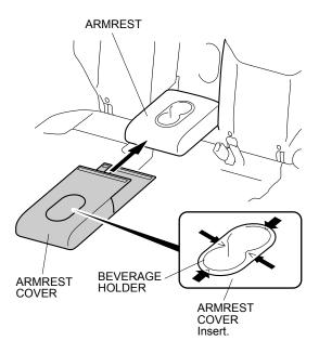
8. Raise the armrest. Pull the armrest cover between the armrest and left rear seat back, and secure the fasteners on the armrest cover as shown.
