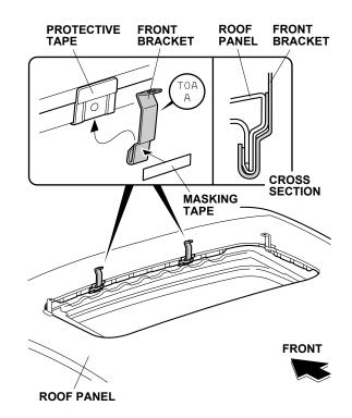
12. Set the moonroof visor on the vehicle roof in front of the moonroof opening, and adjust its position so the holes in the visor are aligned with the holes in the front brackets. Loosely install the moonroof visor to the front brackets with two screws and two nuts. Remove the masking tapes from the front brackets.
