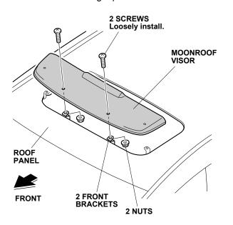
13. Loosely install the moonroof visor to the side brackets with two screws and two nuts. Remove the masking tape from the side brackets.
