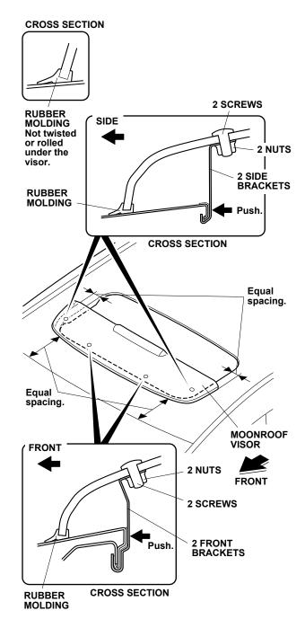
15. Tighten two screws and two nuts on each side of the vehicle first, then tighten two screws and two nuts on the front. Tighten while applying pressure so that there is no gap between the brackets and the roof panel. Torque the screws to 2 N·m (1.5 lbf·ft).
